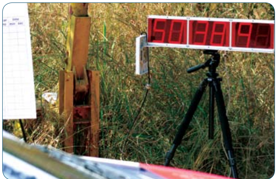
Fig. 2: When in a timing control zone the SafeTrack is connected via the TR radio system to the Rallytime GPS TR in order to identify the car number to the control and receive time information back.
