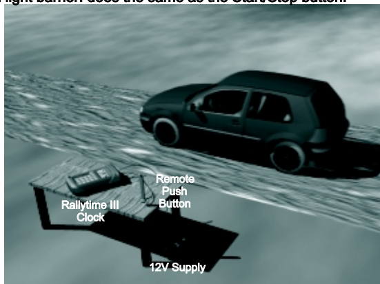
The typical peripheral setup for stop and time controls
